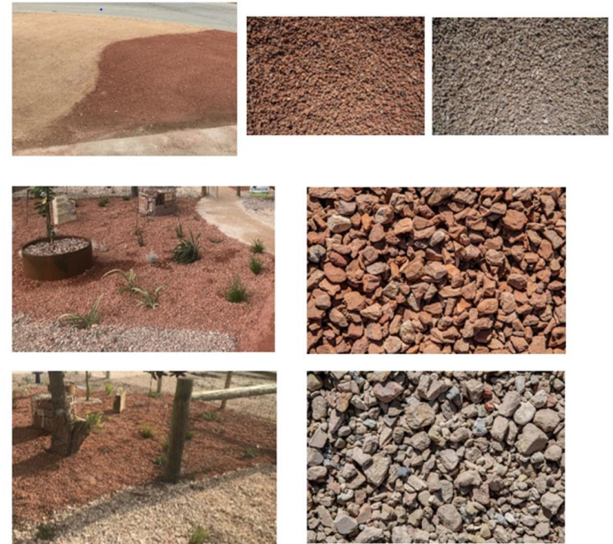
Tree reuse and crushed bricks at Jandakot Fire Station
