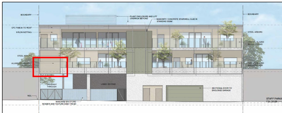
Figure 13 — 2021 Approved Aluminium Louvred Screen (First-Floor West Elevation)
