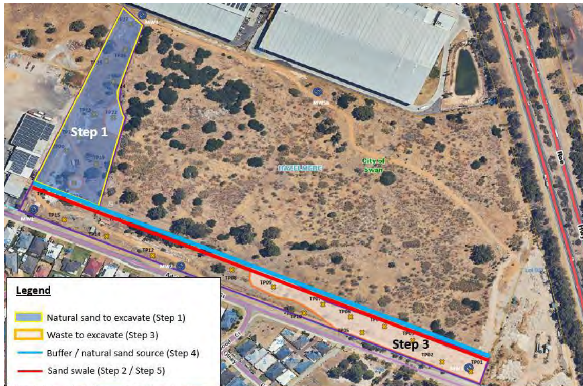
Figure 2 – Illustration of Proposed Remediation Areas and Steps – all locations approximate (Source: RAP, 2025)
